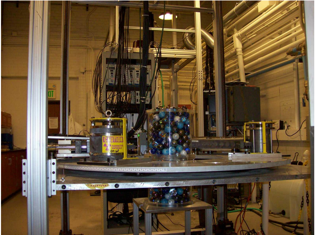
Figure 3.3: Setup of 2 feet pebble bed reactor filled with 2 inch pebble size mounted inside the DSCT technique
