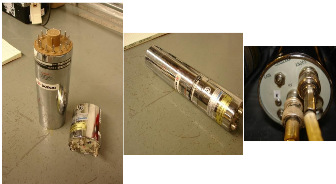
Figure 3.16: The NaI(Tl) solid state scintillation detector assembly
